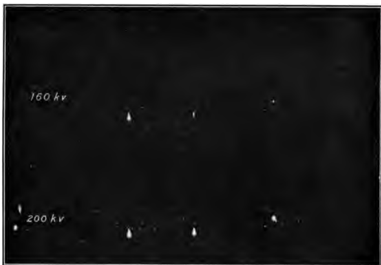
FIG. 67.—Corona on a No. 3/0 line cable. Dry.
